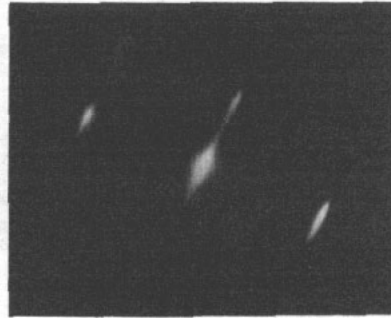
Figure 4. RHEED pattern of the deposited diamond thin-film surface with the beam azimuth [112].
